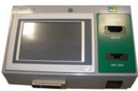
**TED Terminal** is designed for the simple communication of workers in CA with the SEOD system upon their entrance/exit to/from the CA of a nuclear power plant.
