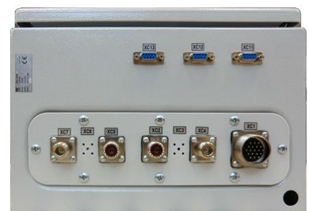
Connectors of the processing coincidence unit (can be modified)
