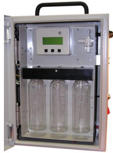
Model V3Ha ( 3 H extraction in the form of H 2 O, compact version)
