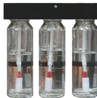
Assembled bottle array for NaOH solution
