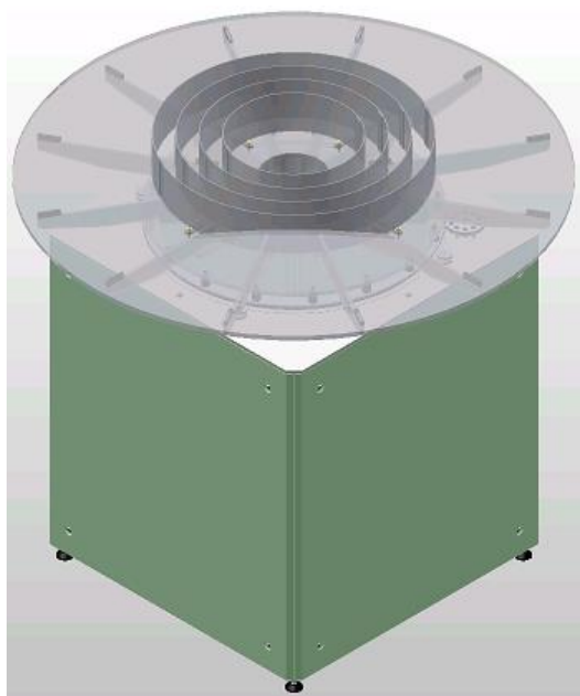
PGI-01 irradiator workplace with rotary table
