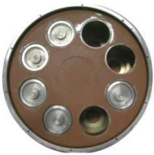
Carousel holder with the sealed sources
