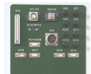
Measuring panel: input-output connectors
