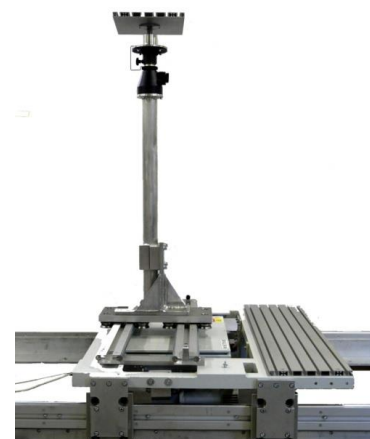
Calibration Bench (a type with one axe motorized movement)
