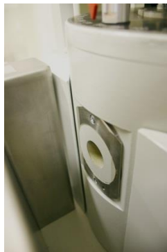
Exchangeable collimator of low sensitivity
